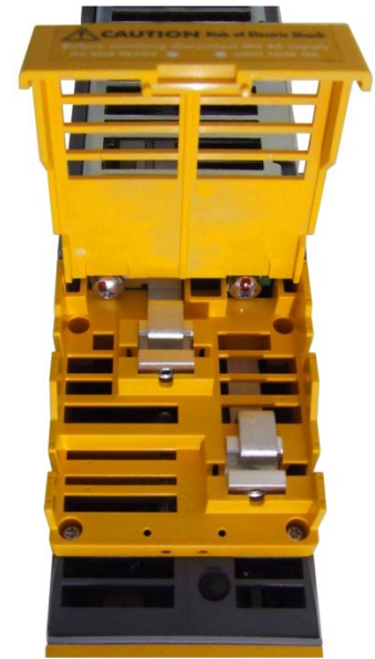
AC890 bus bar connections
